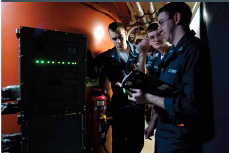
▲ MT3 Colin Costello and MT3 Richard Mullins get some help on understanding missile tube radiation monitoring panels from the missile compartment roving patrol, MT3 Johnathan Pierce. Like all Navy jobs, qualifying for watchstations is a never-ending process.
