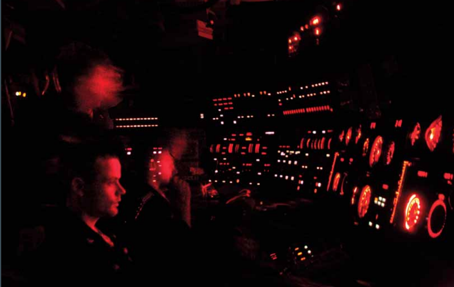
▲ During night surface or periscope operations, submarines rig the control room for red to help maximize their night vision.
